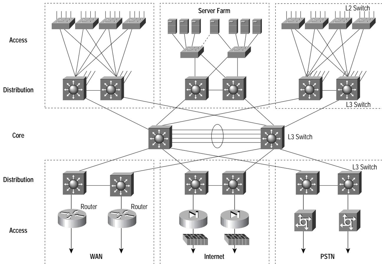
A detailed discussion of the above design is outside the scope of this paper, so the discussion here will be limited to the functionality of the components. As in the branch example, Cisco routers provide the required WAN and PSTN access. Here these routers are required to scale to support the incoming and tandem traffic from many smaller branch locations. Typical platforms used for this function would include the Cisco 7200 and 7500 families of multiprotocol routers.
