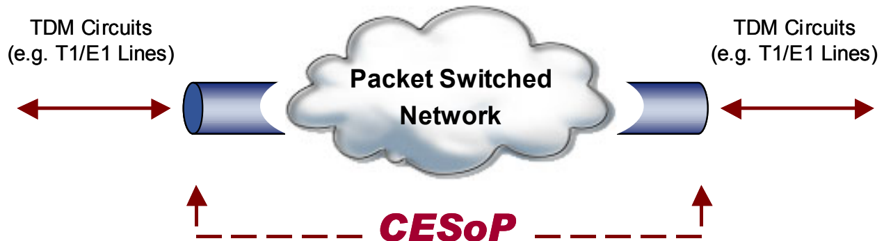
Figure 1 Circuit Emulation across a Packet Switched Network
