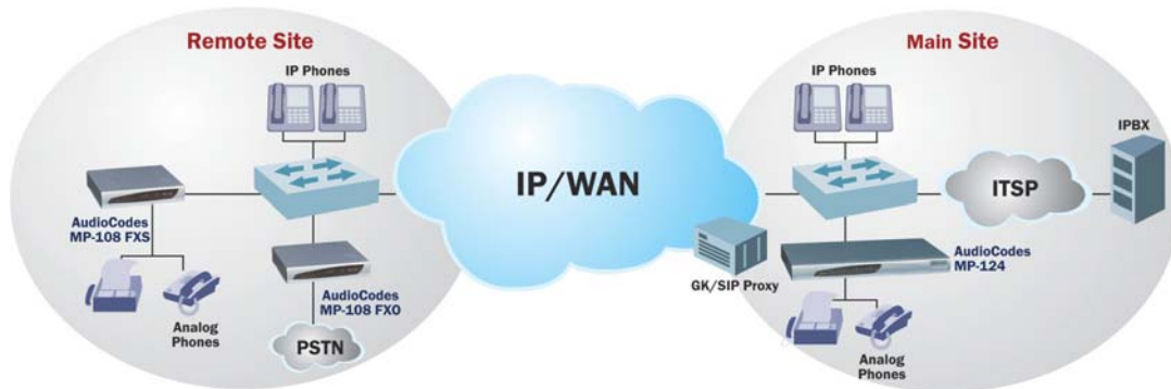
Figure 5 – Support for Analog Devices in iPBX Environment
