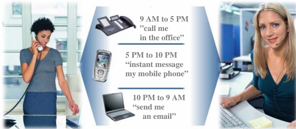
Figure 2: Contact Center Follow up - SIP enables a Personalized Communications Model, via "one number" access to reach any media according to configured rules
